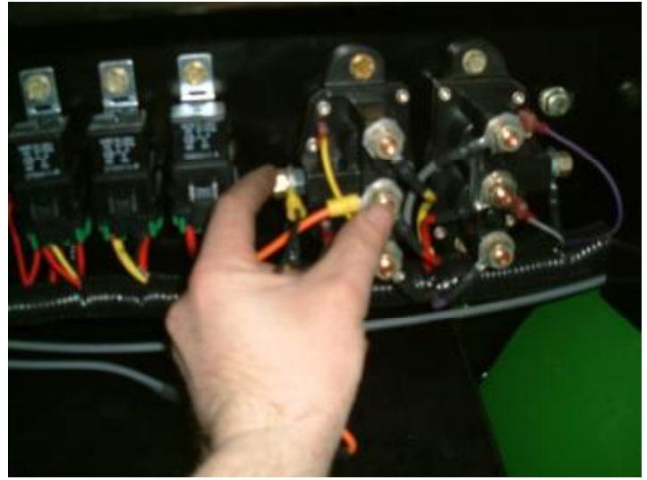
Figure 22: Power wire attachment locations
