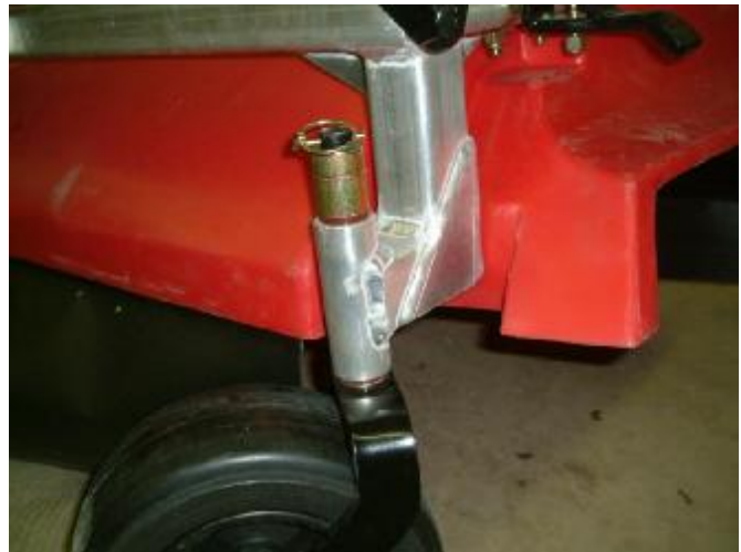
Figure 4: Castor wheel and boom height spacers
