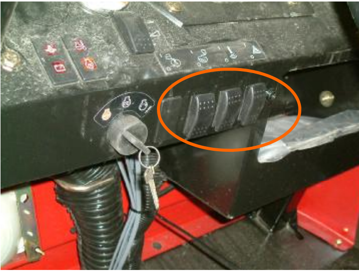
Figure 23: Dash of 5800 with inserted switches
