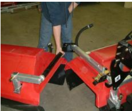
Figure 13: Attaching break away tube to center section
