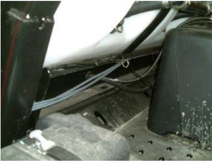
Figure 26: Wire placement along tank
