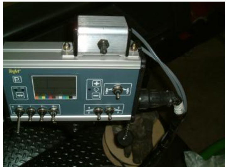
Figure 24: Attachment of center switch box to top of main console
