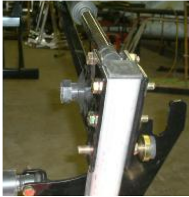
Figure 6: Bolt and wing stop orientation
